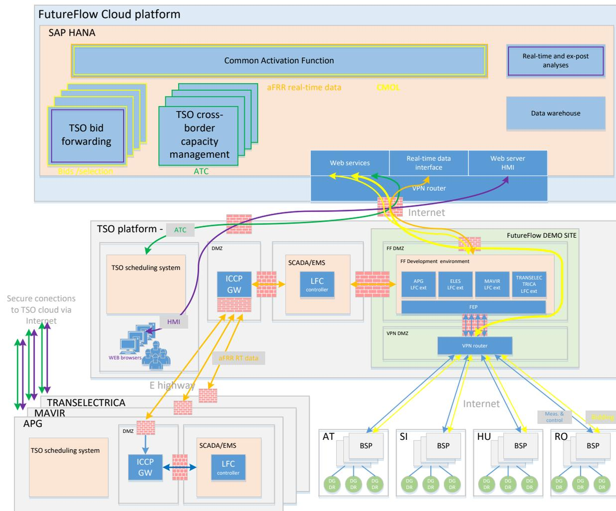
Figure 1: The FutureFlow DEMO Site System Architecture [6]
