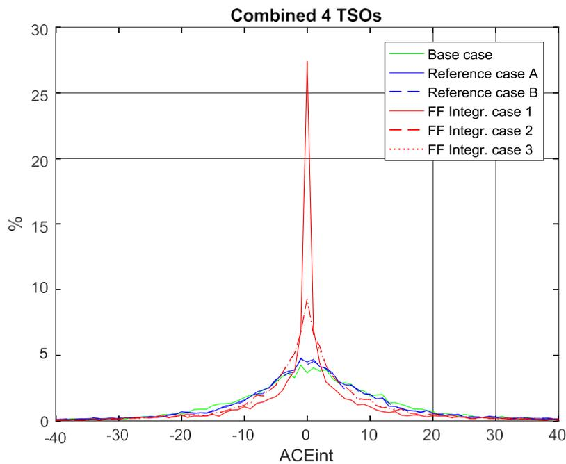
Figure 7: Envelope of 15-min average Area Control Error for each analysed case - all 4 TSOs combined
