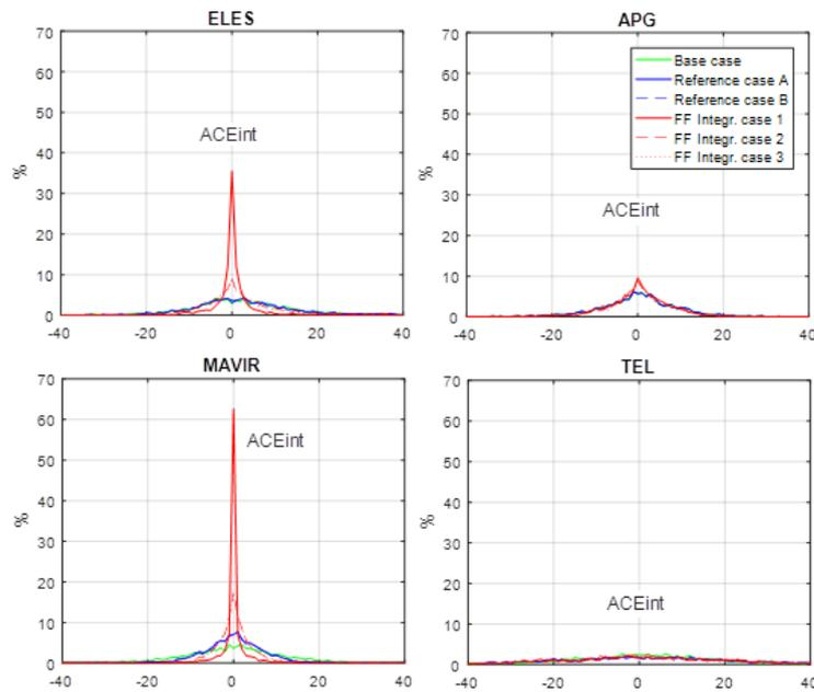
Figure 6: Envelope of 15-min average Area Control Error for each analysed case per TSOs
