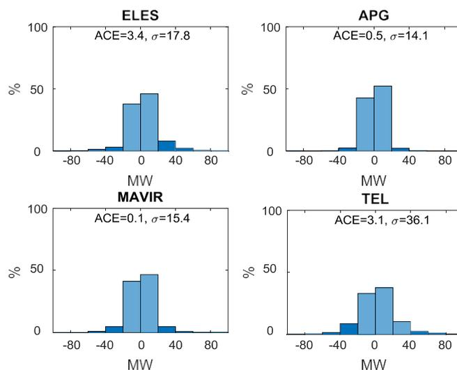
Figure 4: Average Area Control Error per 15 minute  $\Delta P$  [MW] - Class width 20 MW
