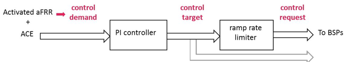
Figure 2: LFC and possible aFRR exchange demand sources: control demand, control target/request
